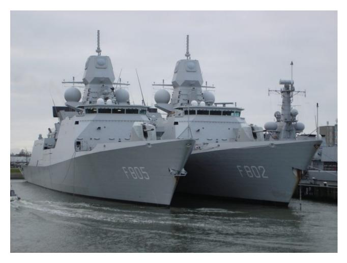
Photo: Dutch frigates with electronic high-tech by Thales Netherlands, including the APAR radar. The APAR is a multifunctional radar that can carry out several tasks simultaneously, such as surveillance and tracking a large number of targets, while aiming missiles.
